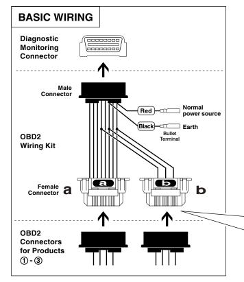
When you wish to use the Diagnostic Monitoring Connector to run diagnostic tests, disconnect the OBD2 male connector and run the tests.
