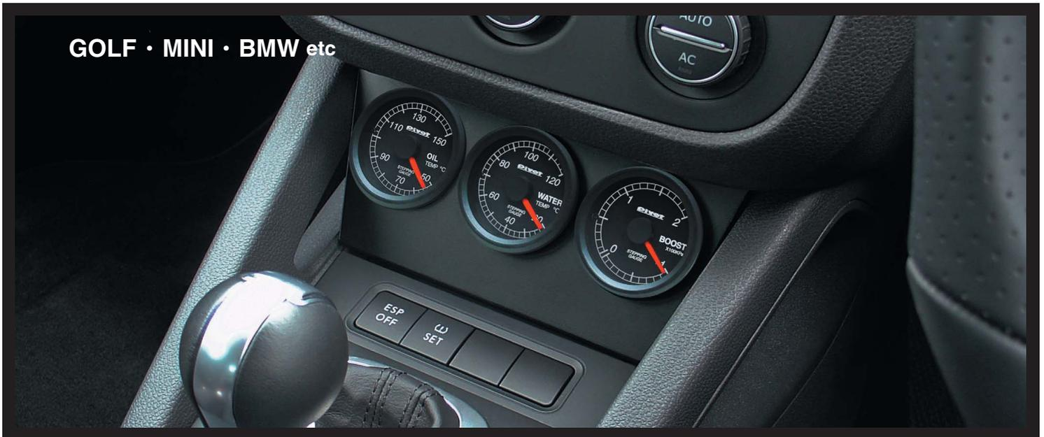
VW GOLF V Triple Gauge Type BOOST, WATER TEMP and OIL TEMP
