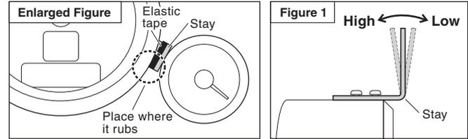
With a little force it is possible to bend the L shaped stay attached to the meter hood. If you wish to adjust the height of the gauge, please bend the stay (figure 1). Please bend only the hood before attaching it to the standard tachometer; bending it after attaching may cause damage to the screw holes if the standard tachometer.
