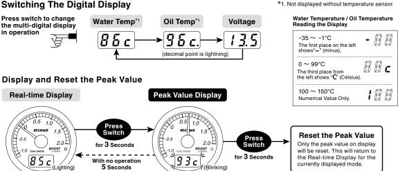
\*Peak readings are reset when the key is turned OFF.
