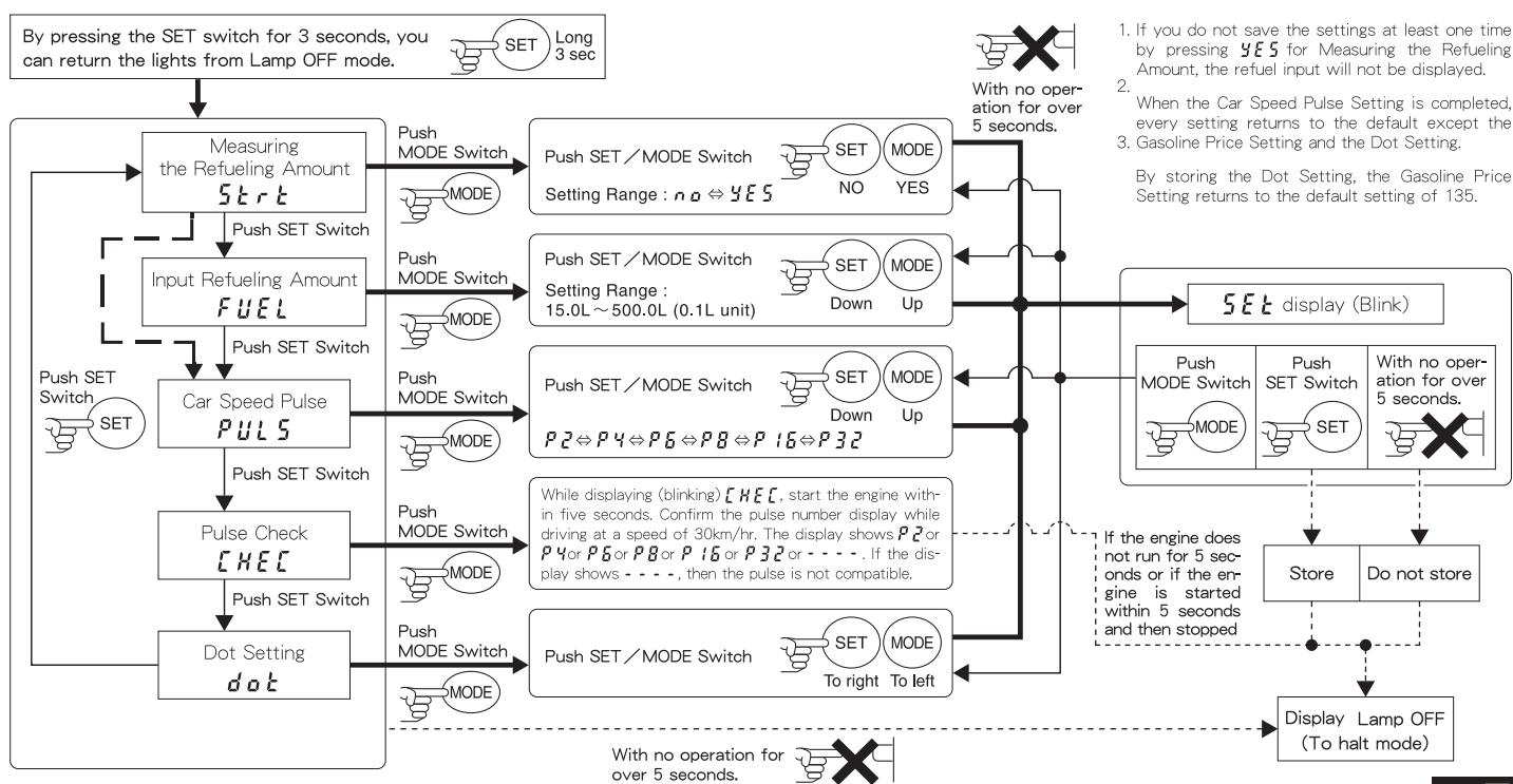
1. If you do not save the settings at least one time by pressing **SEt** for Measuring the Refueling Amount, the refuel input will not be displayed.
