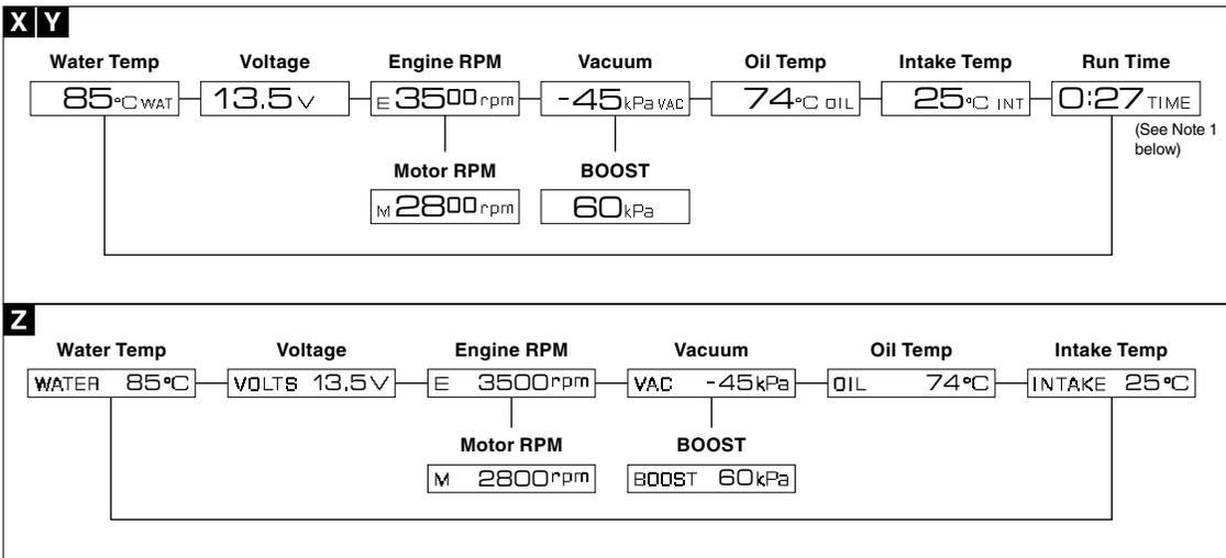
Note 1: Run Time (time elapsed from start of engine) can only be shown in **X** and **Y**, not in **Z**.
