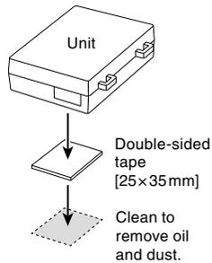
● **When Fastening to a Cable or Pipe**
