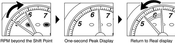
**PEAK** Shows the peak reading after the engine begins running
