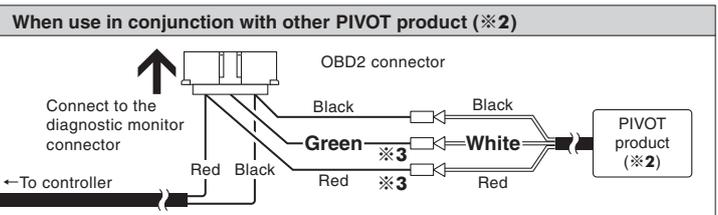
※3 Remove the red and green insulation caps and insert the male connector.
