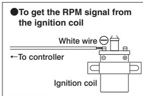
When connecting the RPM signal to the ignition coil or diagnosis and the indicated rpm on the meter may be obviously lower than the actual rpm as shown on tachometer
