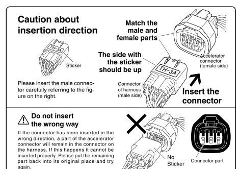
Not to disconnect the connector, fasten by wrapping insulation tape around it.
