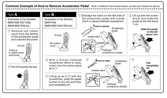
Only disconnect the accelerator connector after having waited at least fifteen minutes from the time that the ignition turned to the OFF position After the engine has been stopped for at least fifteen minutes, pull off the accelerator
