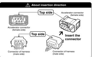
4 Insert the female side of the specialized harness into the male side of the accelerator connector
