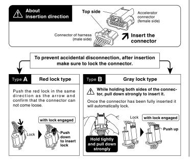
Insert the female side of the specialized harness into the male side of the accelerator connector
