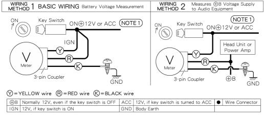
NOTE 1. If it is not necessary to measure peak data (lowest voltage) when starting the engine, connect to ACC.
