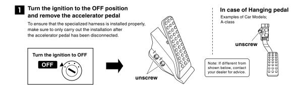
Only disconnect the accelerator connector after having waited at least fifteen minutes from the time that the ignition turned to the OFF position
