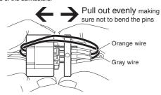
X With the orange and gray wires, which connect the male and female sides of the connector, at the top of the connector pull the connector apart.
