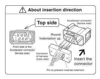
If any of the pins on the male side are bent and cannot be connected properly, correct the bent pins and insert.
